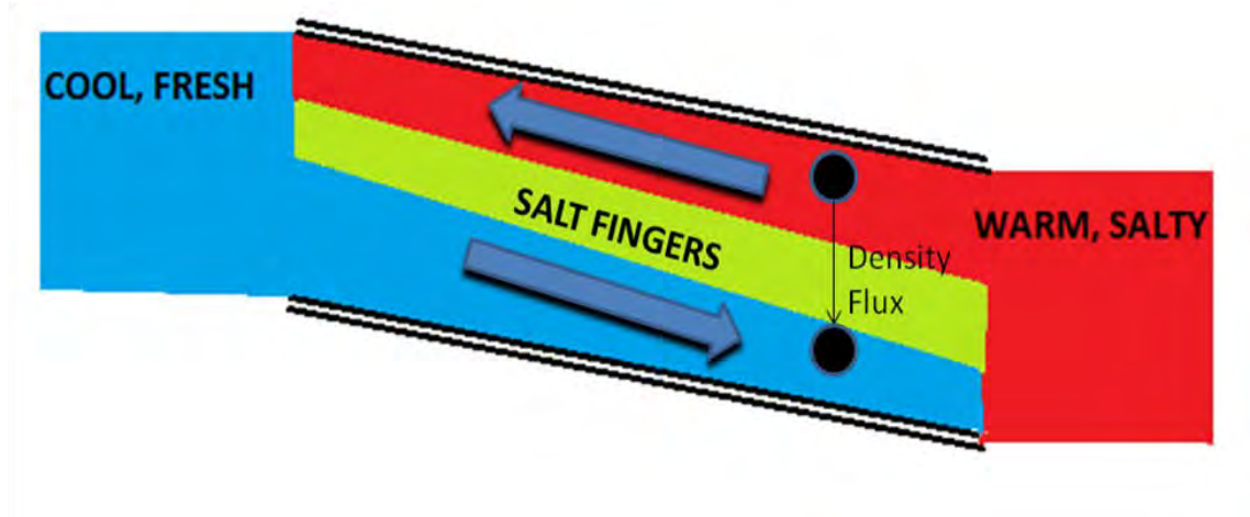
Figure 11. Schematic of a thermohaline front between two water masses. The warm, salty water above cold, fresh creates conditions favorable for salt fingers.
