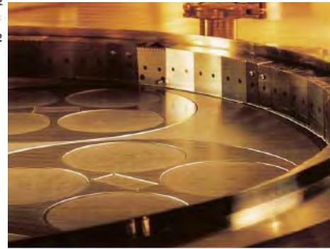
Figure 10. MOCVD multiwafer processing (EENG 596, 2008:slide 13)
