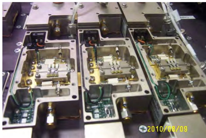
Figure 58. Clamps attached above devices and test modules attached to heater bar
