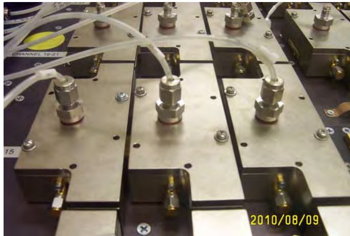
Figure 59. Test module covers and nitrogen tubes attached
