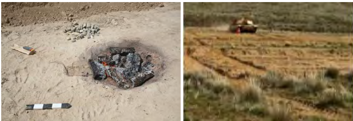
Figure 9. Fire Feature at the Bottom of an Excavated Pit and the M1A1 Tank Driving over the Backfilled Test Pits
