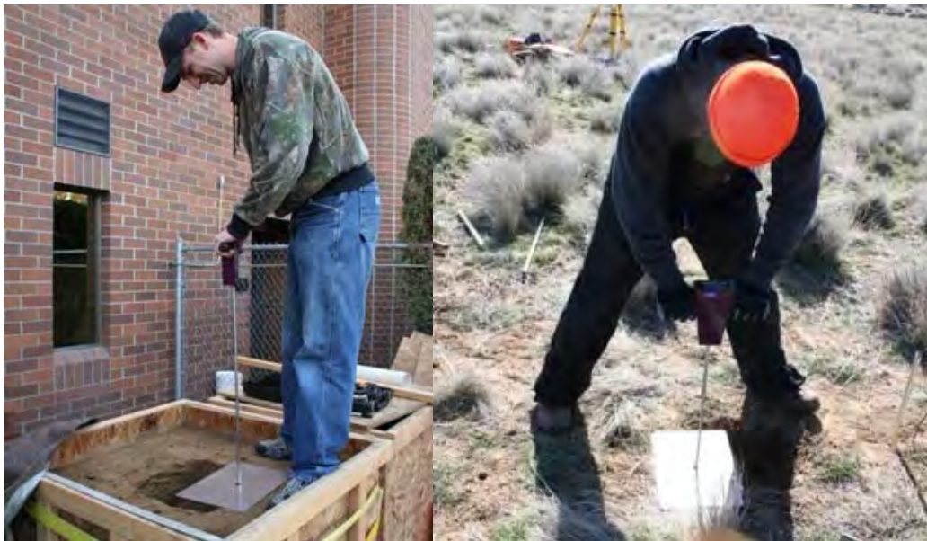
Figure 6. Cone Penetrometer Measurements Conducted in an Engineered Rut and in the Field.
