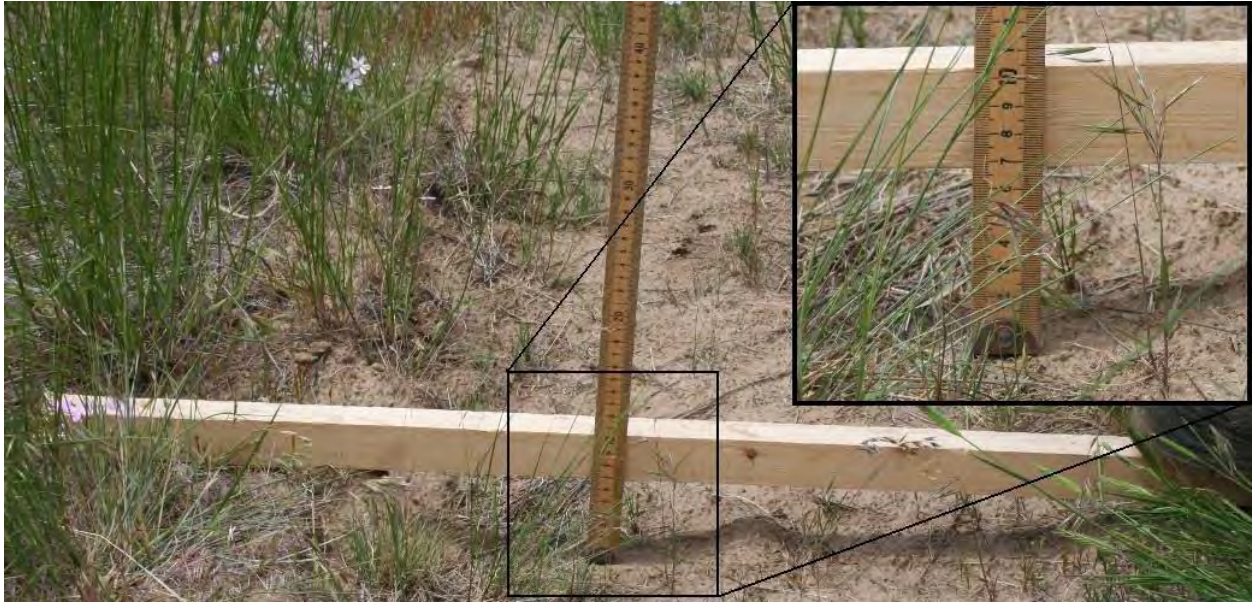
Figure 60. Rut Left in Previously Undisturbed Area by M1A1 Tank After Four Passes
