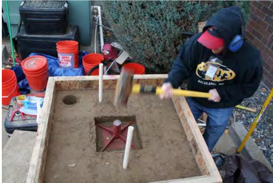
Figure 4. Manual Rut Formation for Box Tests. Note the hole left from the density sample collected prior to compaction and the PVC sleeves for down-hole magnetic susceptibility measurements.
