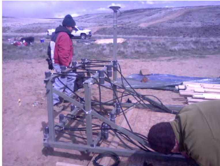
Figure 12. Magnetometer Data Collection Cart Used at the Drive-Over Test Site
