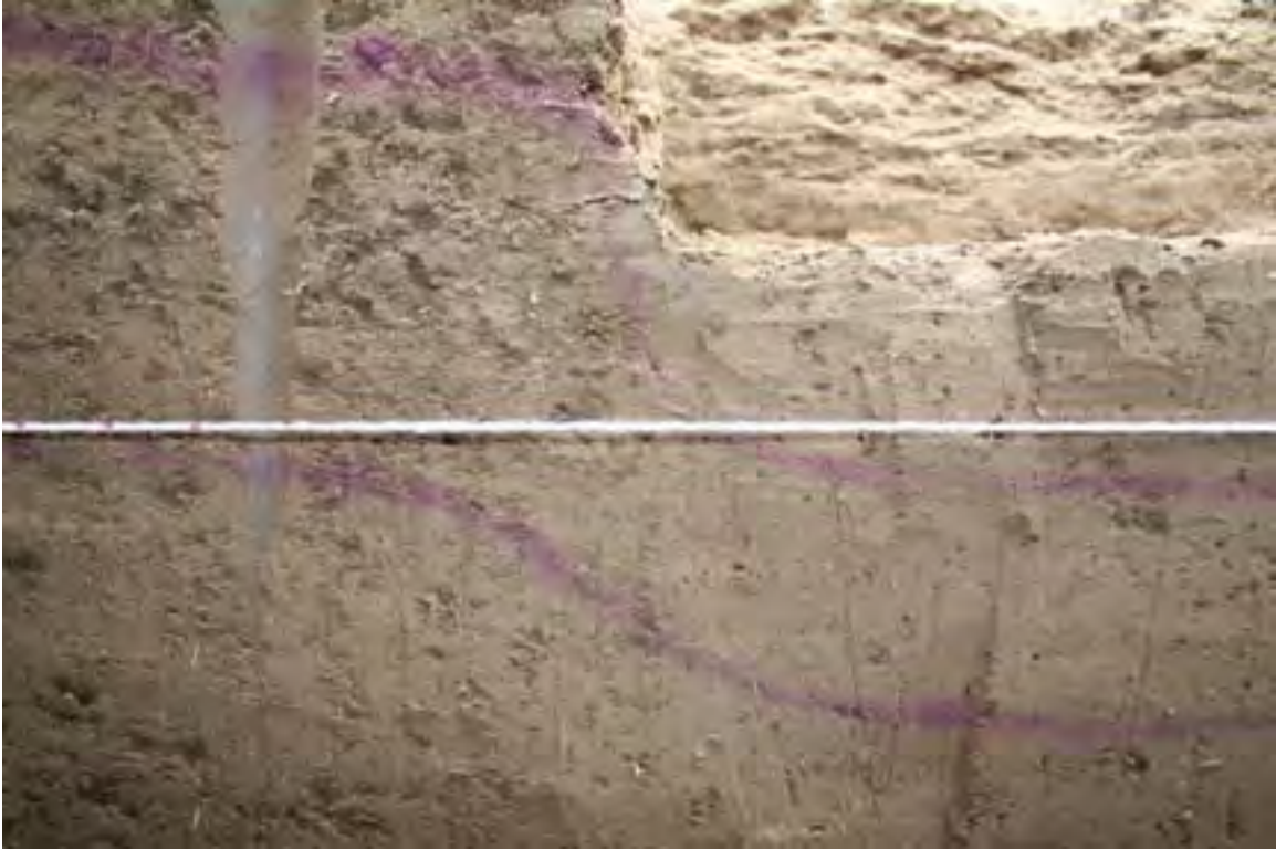
Figure 33. Close-Up View of the Dyed Soil Layers, and the Deformation Caused by Compaction During the Second Box Test
