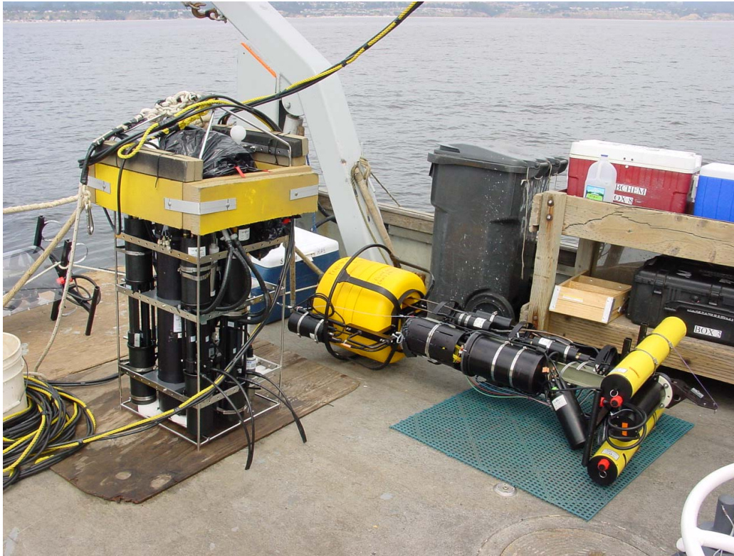
Figure 1. The autonomous URI IOPC profiler (on the right) with the APNA II nutrient analyzer payload and the URI High Resolution Profiler (on the left), with a SubChemPak Analyzer payload. [The URI High Resolution Profiler is a cabled, ship-deployed instrument that uses buoyancy adjustment to descend slowly through the water column while it measures a variety of physical, biological, optical and chemical properties of the water. The URI IOPC profiler is an autonomous, battery operated moored-profiler that may be deployed in the coastal ocean for weeks at a time. It contains a full suite of instruments and sensors for monitoring the physical, optical, biological and chemical properties of the water. The profiler can be programmed to make repeated profiles, from the bottom to the surface, on a pre-set time schedule, to send the results by radio telemetry to a shore- or ship-based receiver station, and then return to the bottom to wait for the time to start the next profile.]
