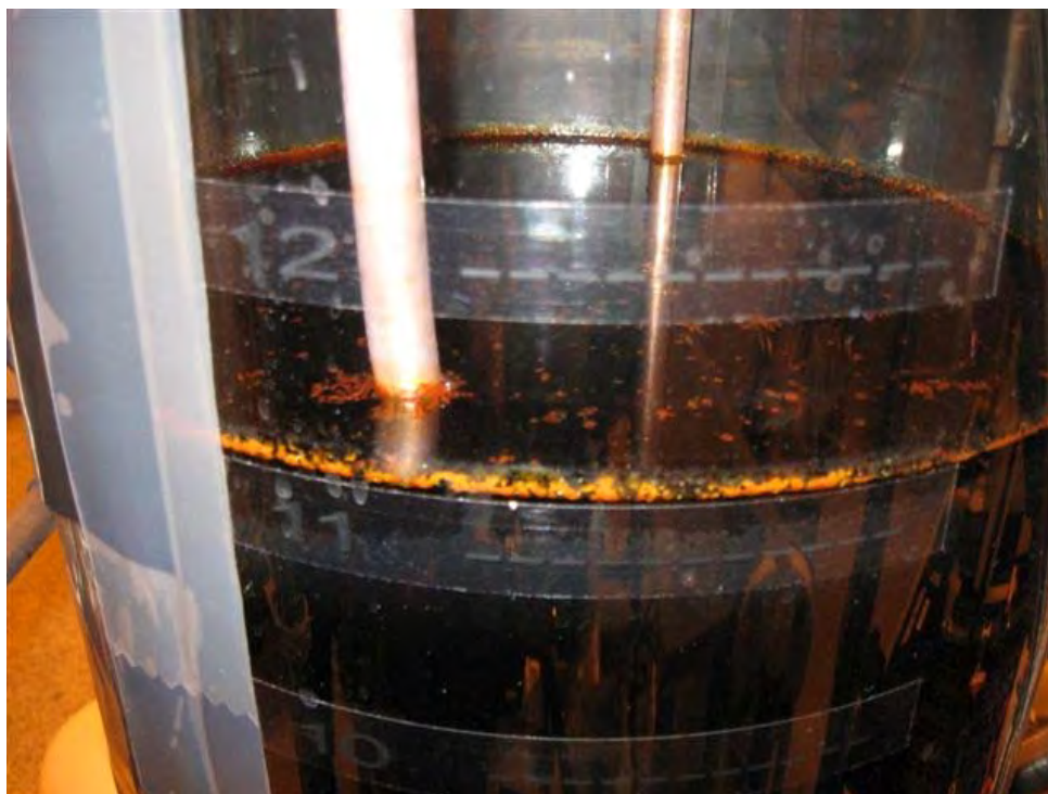
Figure 9. Orange gummy by-product in analyte vessel following Run 3.
