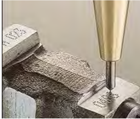
Figure 37. Marking ID Numbers via Dot Peening. Taken from the Website of DAPRA, a Provider of Dot Peening Equipment. www.dapramarking.com/dot-peen-marking
