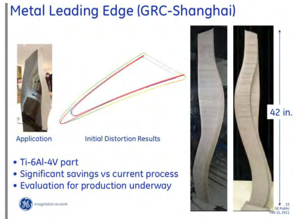
Figure 10. 42” Jet Engine Fan Blade – GE Research - Shanghai
