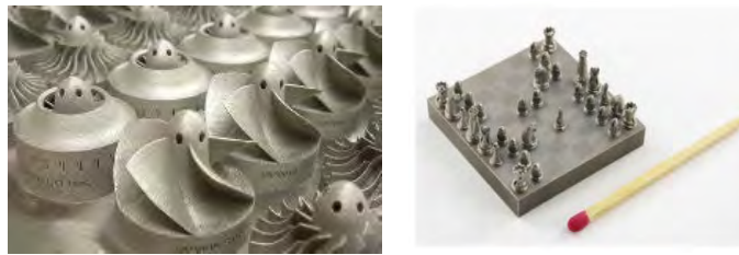
Figure 4. Examples of Components Fabricated Using DMLS (www.electrooptics.com, www.eos.info)
