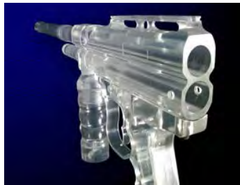
Figure 19. Part Fabricated Using Stereolithography
