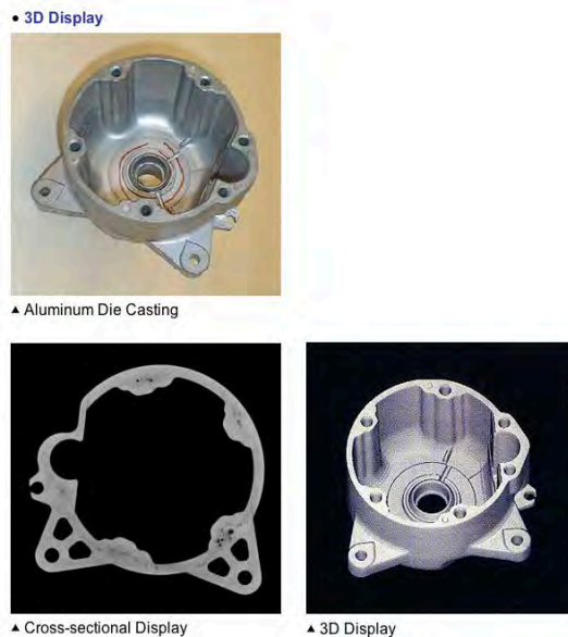
Figure 56. Industrial CT Scanning of Aluminum Cast Part ( www.toshiba-itc.com )
