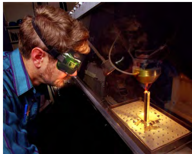
Figure 6. Laser Engineering Net Shaping (LENS) in Process (www.sandia.gov)
