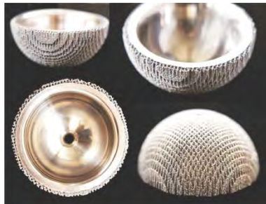
Figure 11. Hip Implant Components Fabricated Using EBM (www.arcam.com)
