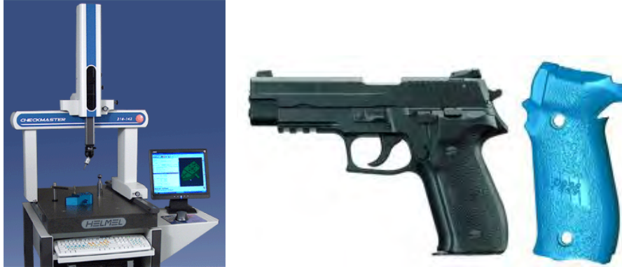
Figure 42. A Table Top CMM (left) and Example of a Point Cloud (Blue) Generated for a Component of a Larger Device. (www.cmmquarterly.com)
