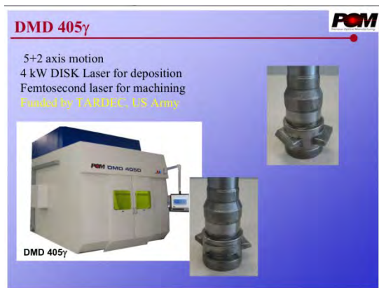
Figure 8. POM DMD System Combined with Subtractive Femtosecond Laser Processing
