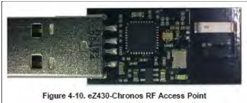
Figure 1. The 915-MHz RF access point photo 14x45 mm (from the TI Chronos User's Guide).
