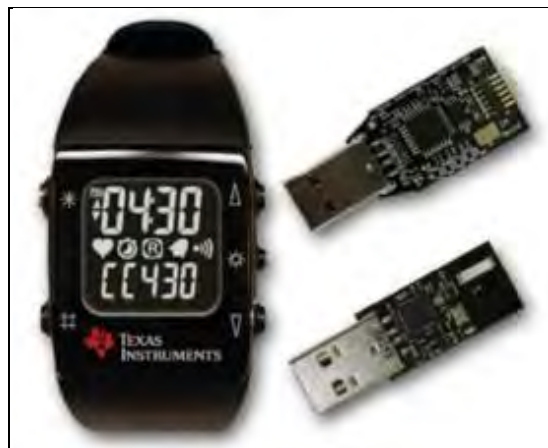
Figure 33. TI Chronos wireless communications development kit.
