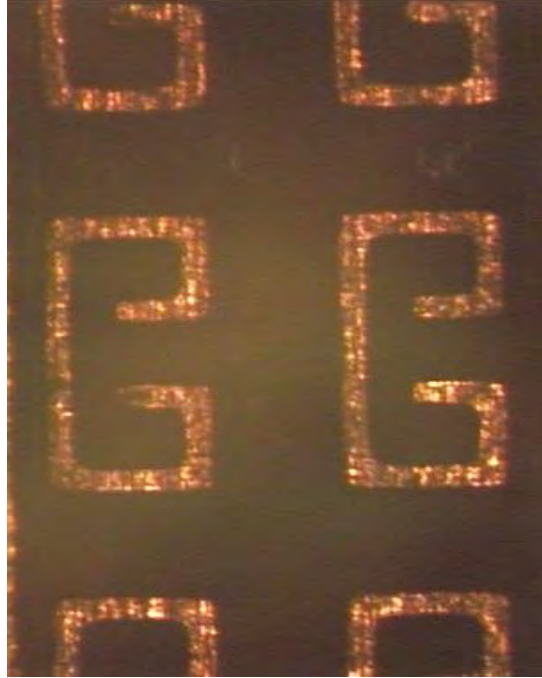
Figure B-2. A close-up view of the fabricated split ring on the Rogers 5870 dielectric material.
