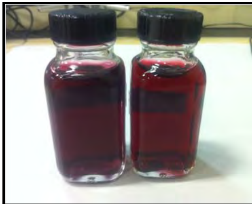
Figure 6. Au nanoparticle solutions after boiling for 15 min.
