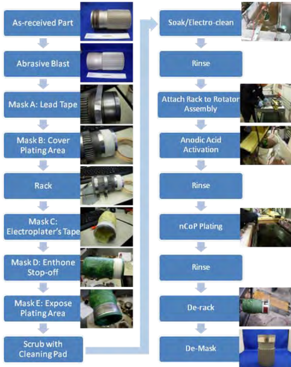
FIGURE 11. PROCESS FLOW CHART FOR J52 SHAFT OD PLATING.
