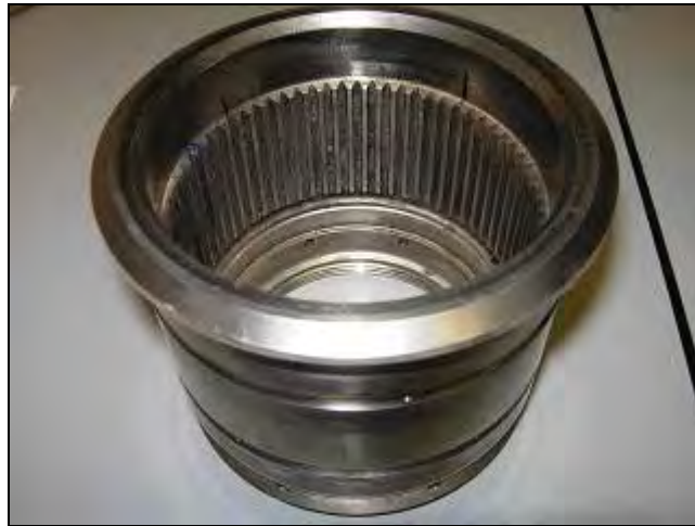
FIGURE 8. J52 COUPLING USED FOR THE INNER DIAMETER PLATING DEMONSTRATION.
