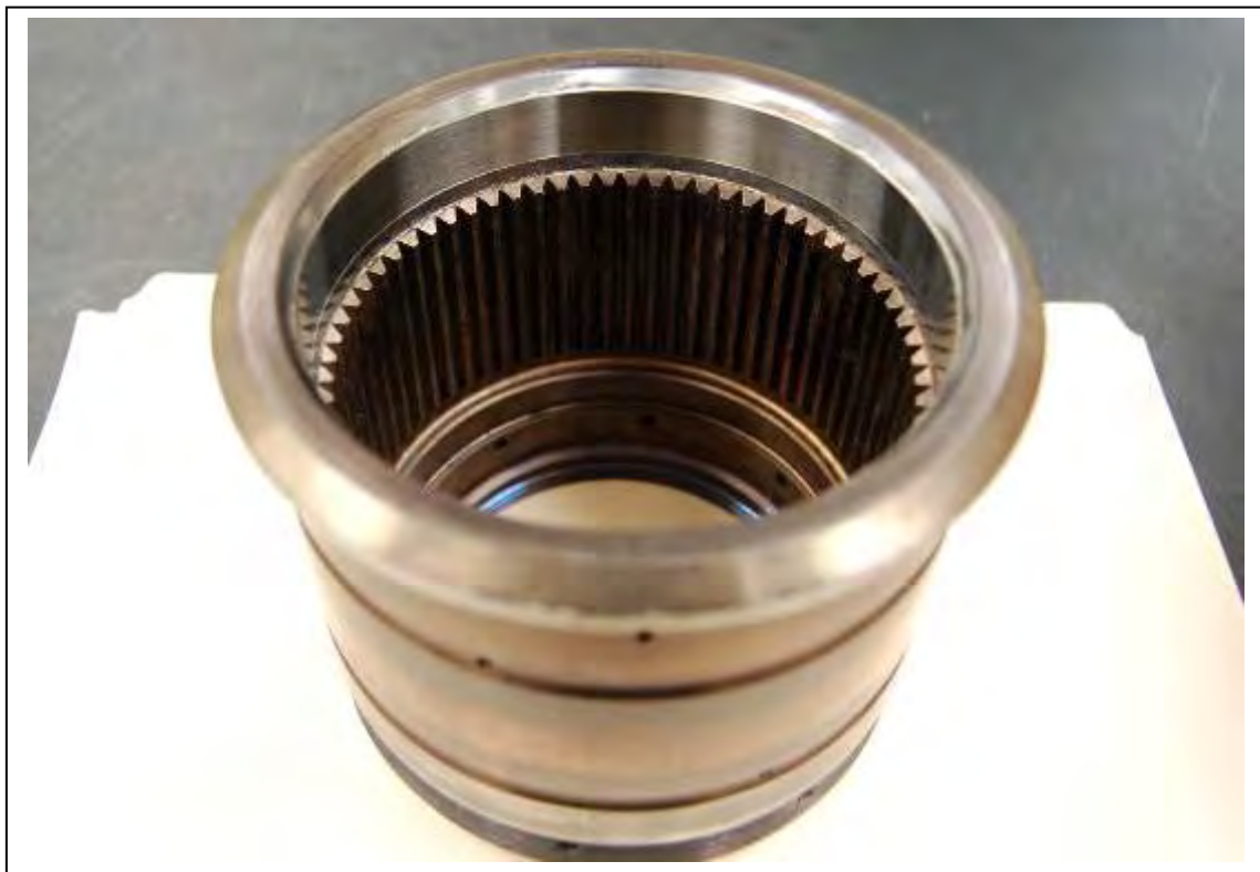
J52 COUPLING FOLLOWING FRC-SE MACHINING OF ID PLATED AREA
