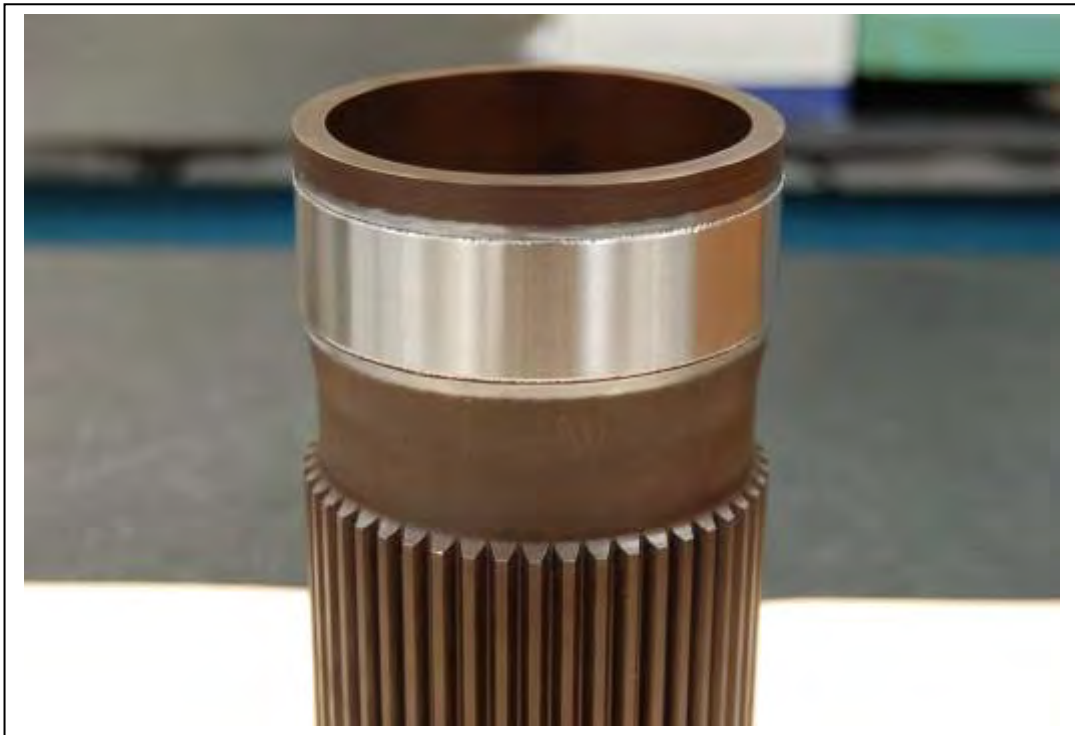
J52 SHAFT SECTION FOLLOWING FRC-SE MACHINING OF OD PLATED AREA
