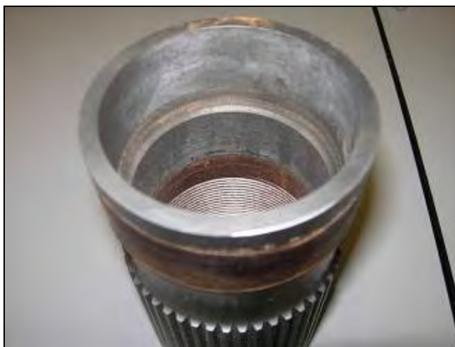
FIGURE 10. J52 SHAFT (SECTION) USED FOR THE OUTER DIAMETER PLATING DEMONSTRATION.
