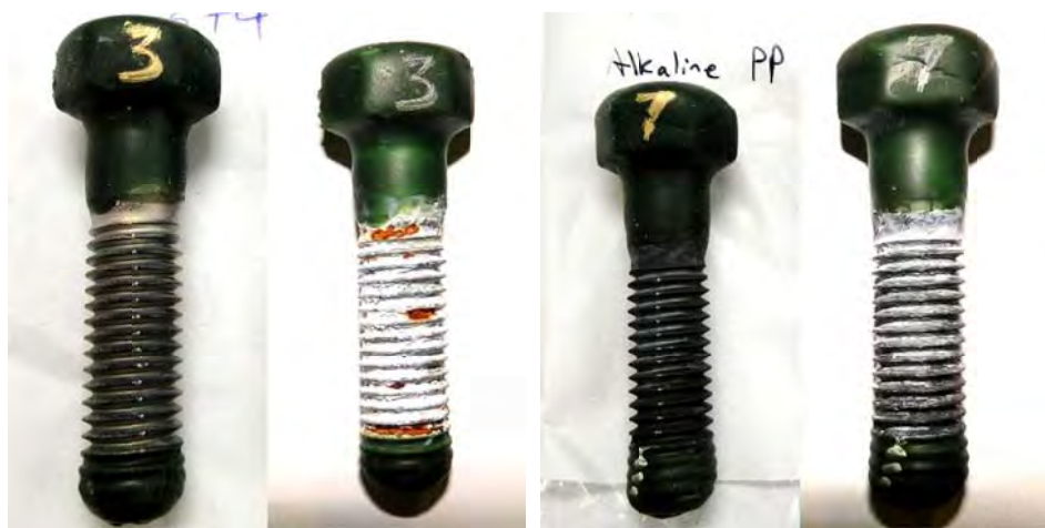
Figure 24: Plated fasteners before and after ASTM B117 testing: Zn-Ni acid PP (left) and Zn-Ni alkaline PP (right). All Zn-Ni acid fasteners showed red rust formation after ~700 h, independent of scribing.
