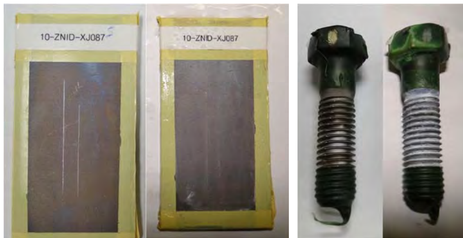
Figure 25: Scribed pulse-reverse plated samples using the Dipsol alkaline system, before and after 1000 h of exposure. Left set: corrosion plaques with minimal white rust formation beginning at ~800 h. Right set: fasteners, both displaying minimal white rusting, independent of scribing.
