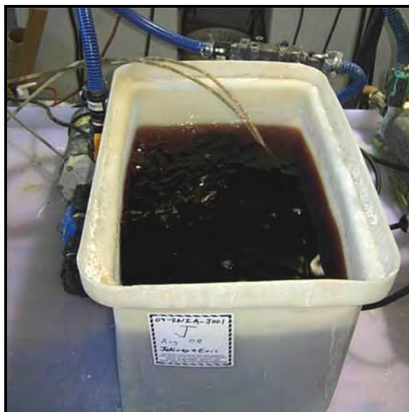
Figure 4: Image of 40 L (10.5 gallon) Zn-Ni alkaline plating set-up.
