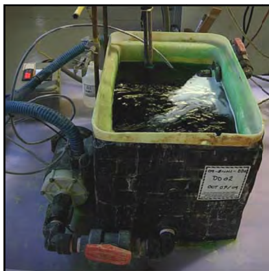
Figure 8: Image of 40 L (10.5 gallon) Zn-Ni acid plating chemistry.
