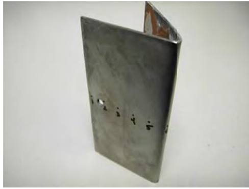
Figure 12: Angled cathode used to investigate plating uniformity between DC and pulsing approaches.
