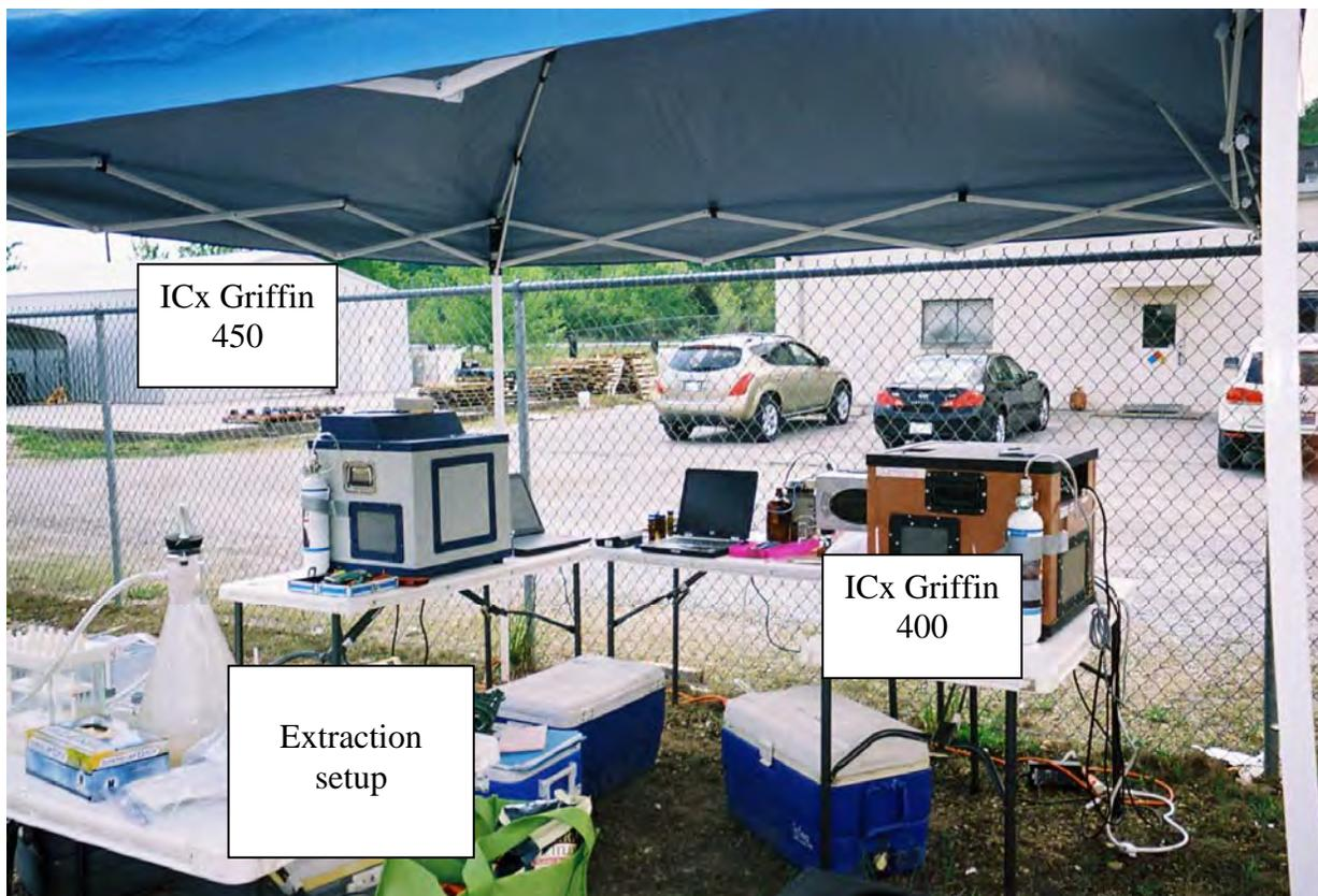
**Figure 2. Field setup for the ICx Griffin 400, the ICx Griffin 450, and the extraction setup.**
