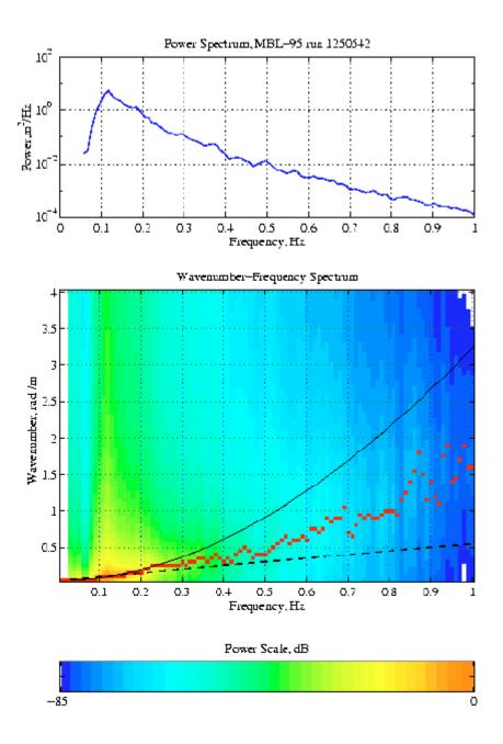
Figure 1. Frequency power spectrum (top) and wavenumber-frequency spectrum (bottom) from the MBL experiment. Run 1250542. Solid line corresponds to the linear dispersion relation. Dashed line corresponds to the propagation speed of dominant waves. Red squares indicate the spectral peak in wavenumber.
