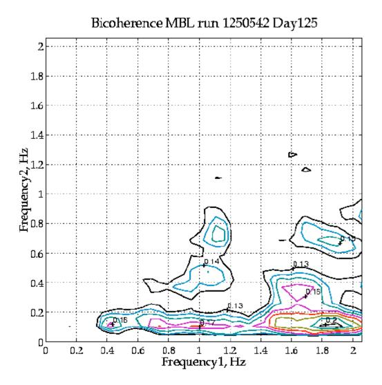
Figure 2. Bicoherence function from the MBL experiment. Run 1250542. Contour levels are every 0.02 of the bicoherence value.
