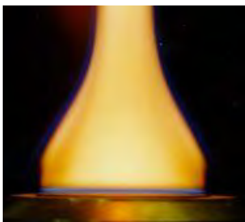
Figure 2. Photograph of typical sooting ethylene premixed flat flame, stabilized on a McKenna burner.
