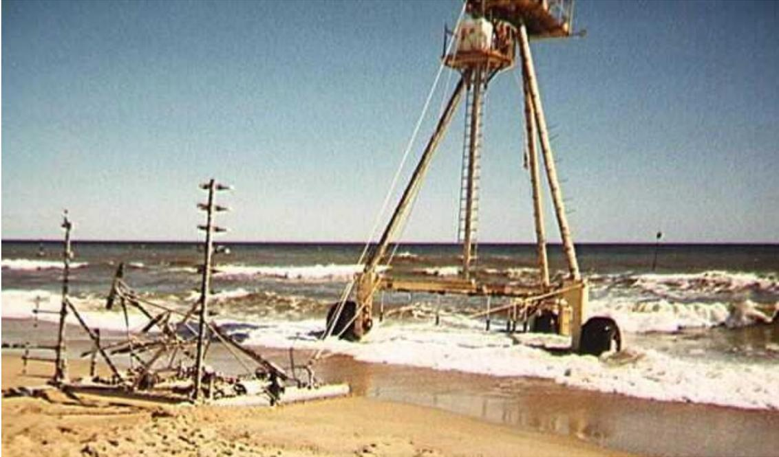
***Figure 1. Instrumented sled (conductivity array on right tower, em current meter array on left tower, BCDV mounted on hydraulically controlled boom at back left) being pulled offshore with instrumented CRAB (acoustic altimeter array along back).***
