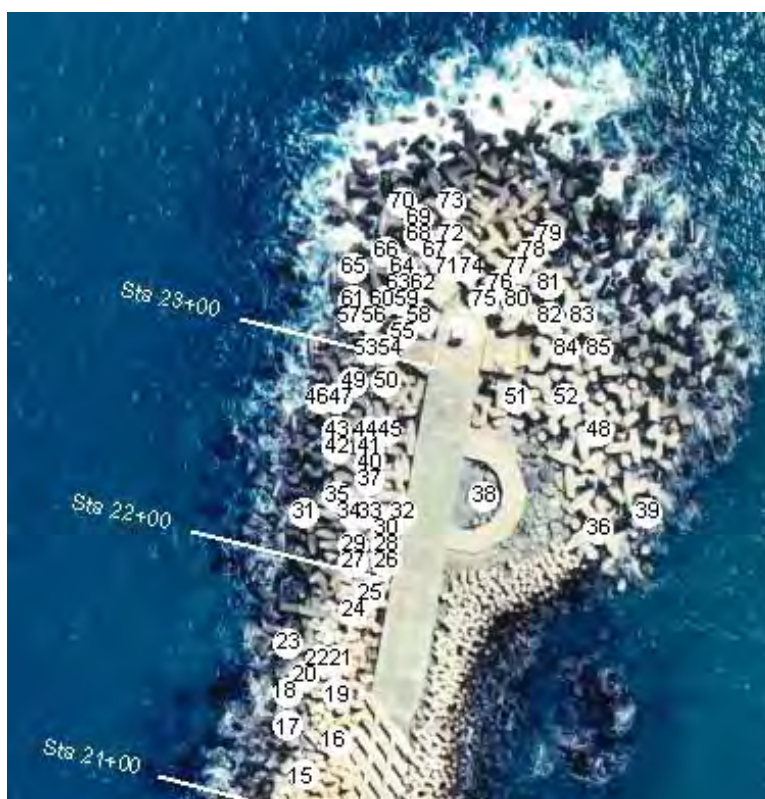
Figure 33. Approximate damage locations on Kahului West Breakwater, photograph 1.
