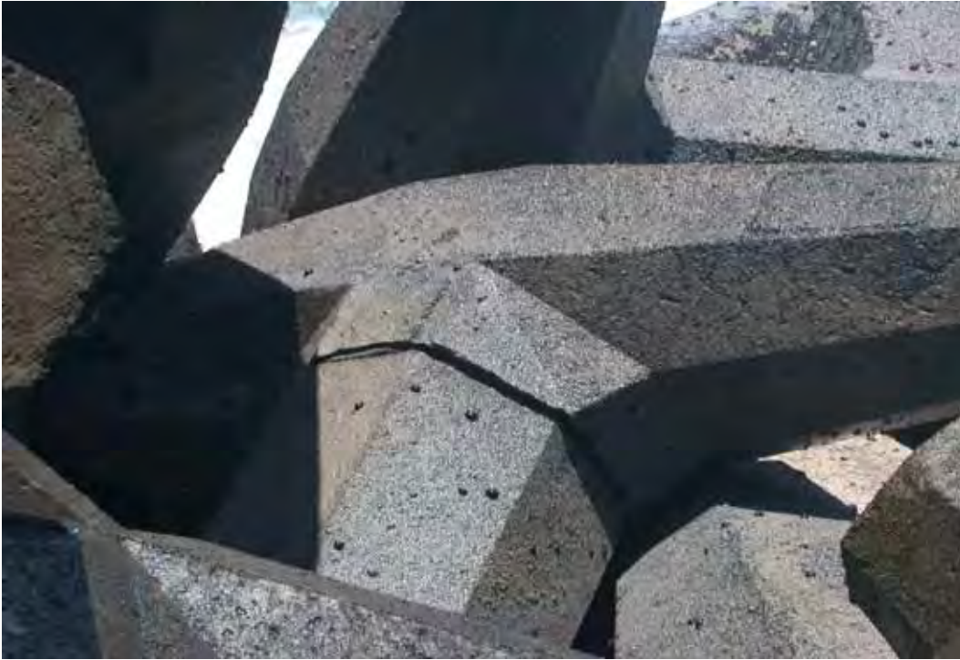
Figure 25. Typical dolosse shank-fluke break.
