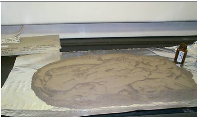
a. The ground sample is spread evenly to a thickness of about 1 cm over a flat surface
