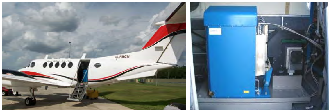
Figure 2. Beechcraft King Air 200 (left) and CHARTS instrument in the aircraft (right).
