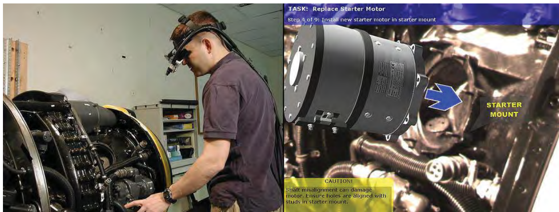
Figure 77: A military mechanic wearing a tracked head-worn display performs a maintenance task on a Rolls Royce DART 510 Engine (Left). A view through the head-worn display depicts information provided using augmented reality to assist the mechanic[116] (Right).
