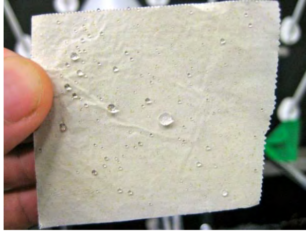
Figure 21: Small water drops stick to the surface of the third sample when tilted vertically (90°). This shows that the surface has been worn to some extent since this behaviour is not seen on the first or second sample. The drops stick to the surface because of the changes in the topography of the sample's surface and perhaps also because of the creases created (and visible) from when the sample was stomped on.
