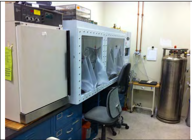
Figure 7: Biospherix instrumentation. It consists of two bays (manipulation and imaging) and atmosphere controlled modules located within a standard warm temperature incubator.
