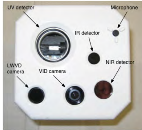
Figure 1. Front view of the Canadian Demonstrator Prototype volume sensor suite (VSS) showing the apertures for the various sensors.
