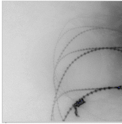
Figure 3. Range image of mine simulant surrounded by concertina wire. Range was 17 feet to the mine in turbid water with c = 0.65 \text{ m}^{-1} .
