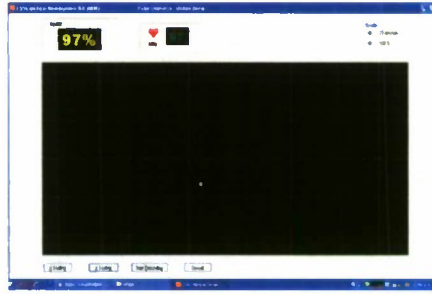
[Figure 6. Computer board output from sensor and LEDs when placed on the finger of a human. Calibration experiments are on-going to define the relationship between output and oxygen saturation in live animals from 100% to 0% O 2 saturation]
