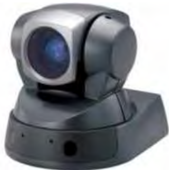
Figure 2. Sony EVID 100 Pan tilt HD Camera for Face Recognition
