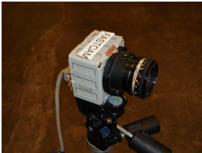
Figure F.15: FASTCAM 1280 PCI shadowgraph camera
