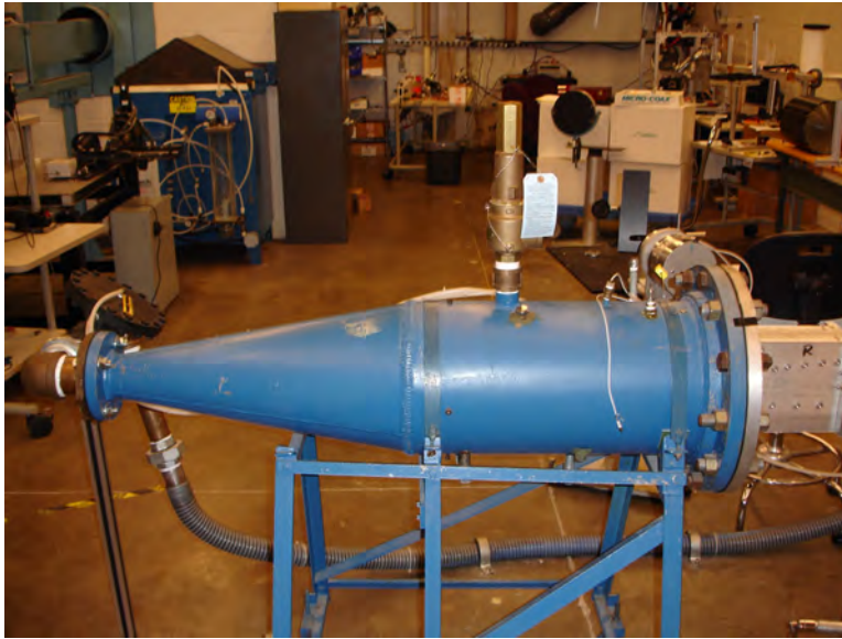
Figure F.11: Stagnation chamber
