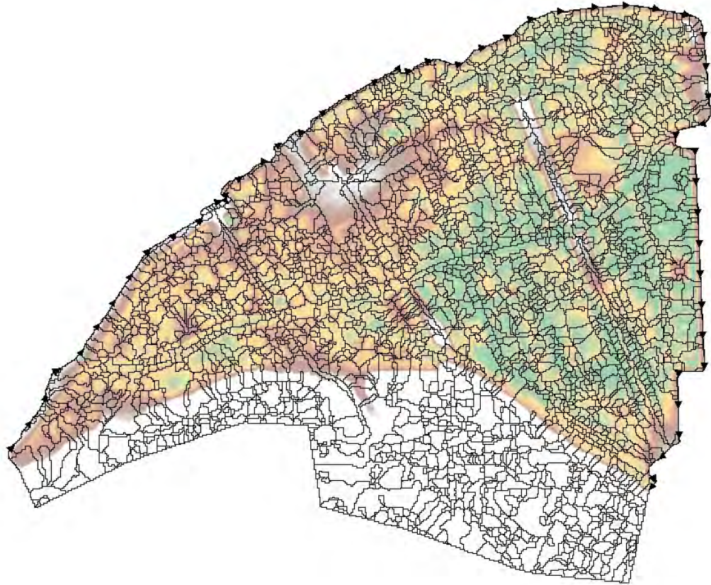
Figure 2 Computational mesh of the Inundation model for the study area.
