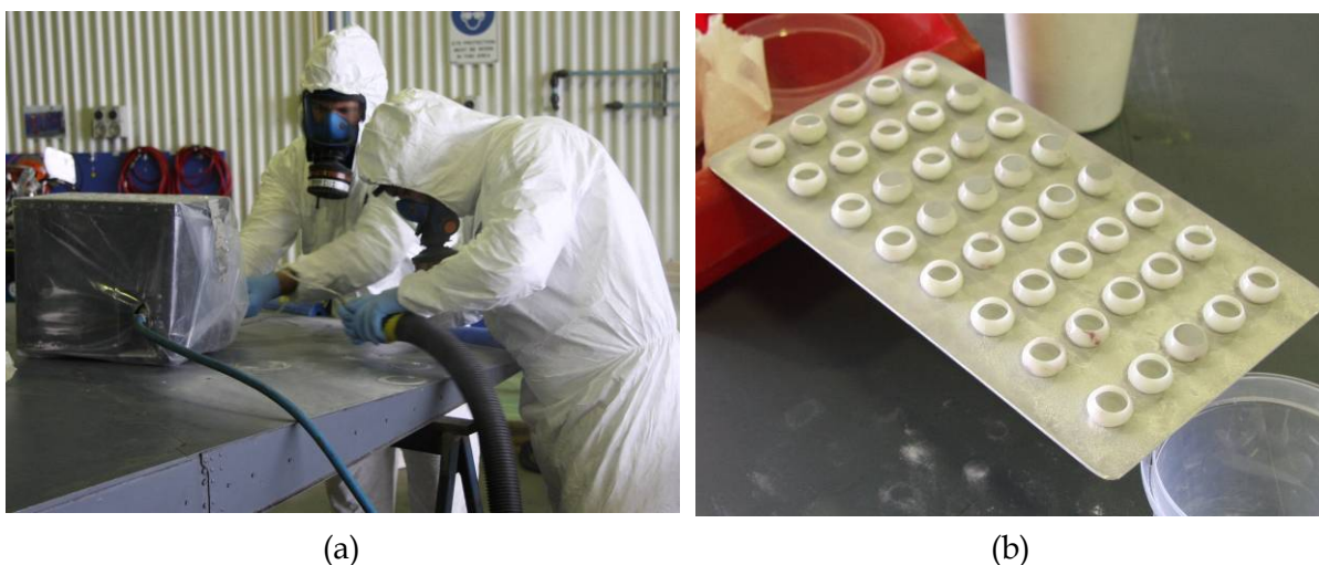
Figure C.8: Photographs showing (a) grit blasting and (b) of a batch of 40 stubs with Teflon ferrules
