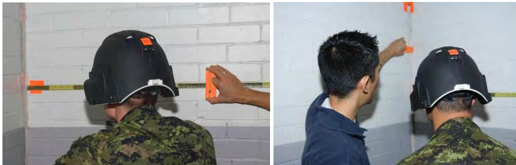
Figure 29: Horizontal (left) and Vertical (right) FOV
