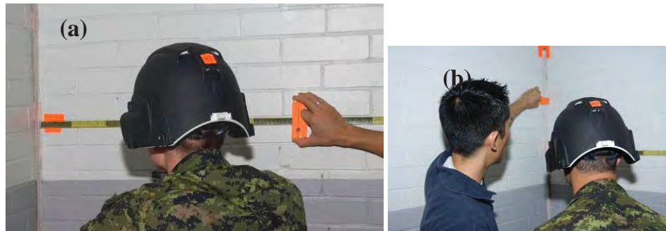
Figure 16: (a) Horizontal and (b) Vertical FOV
