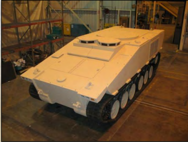
Advanced Reconfigurable Spaceframe (AReS): TARDEC Demonstrator
