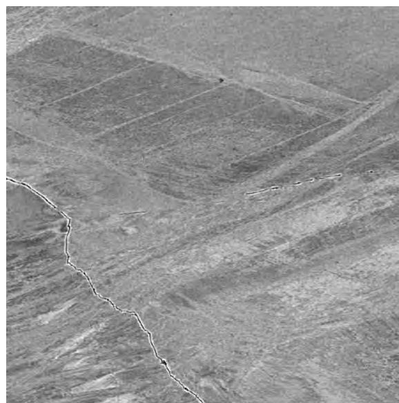
Figure 4. SEM backscatter images of a radial cross-section of a specimen after 60% compression at 23°C.
