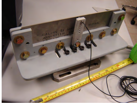
Figure 1: Fixture Mounted to Kistler Dynamometer. Eddy Current Sensors can be Placed at Different Vertical Positions with Increments of 6.35 mm and Five Different Horizontal Locations. Machining Occurs on the Opposite Side of the Plate.
