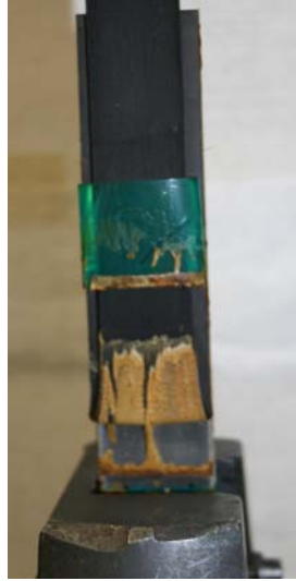
Figure 2. Al-7075 and neoprene rubber substrate.
