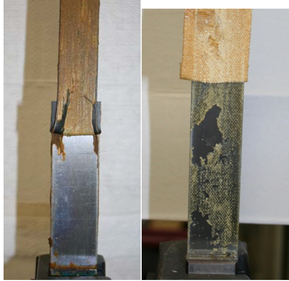
Figure 5. Adhesive failure to Al-7075 substrate (left) and cohesive failure (right).
