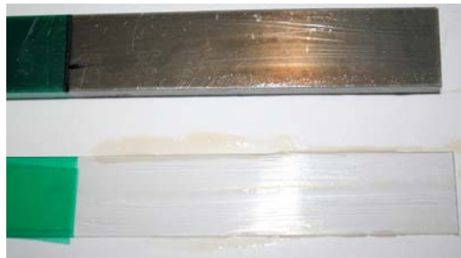
Figure 3. Al-7075 and vinyl plastic substrates coated with adhesive.
