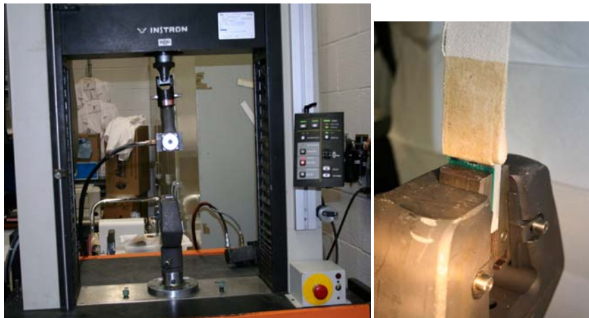
Figure 4. Instron model no. 1123 (left) and stationary lower wedge grip (right).
