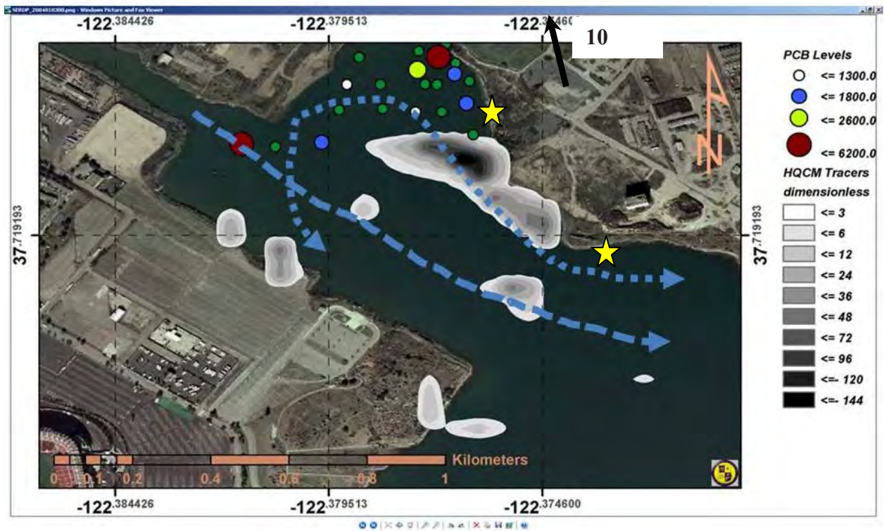
FIGURE 2. Summary of currents and tracer predictions for SE wind event during a tidal cycle on 8-9 January. The maximum tidal outflow is 20 cm/s (long dashed line) and tidal inflow/outflow is 6 cm/s (short dashed line). The wind speed is labeled and the direction is indicated by the arrow. The tracer concentration is contoured after 24 h of release from the locations indicated by stars (dimensionless). The measured concentration of PCBs ( \mu\text{g}/\text{kg} ) is indicated by the solid circles (Battelle et al., 2002).
