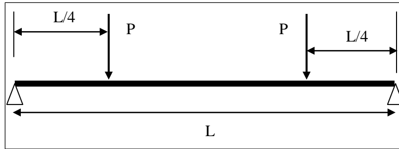
Figure 16. Point loads acting during the pre-flexion process.
