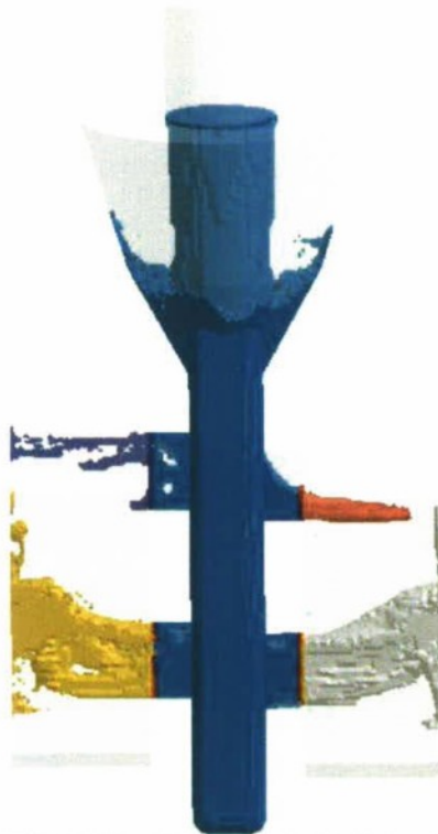
Figure 5 Fluid fill at 307 ms (33% filled) into filling.
