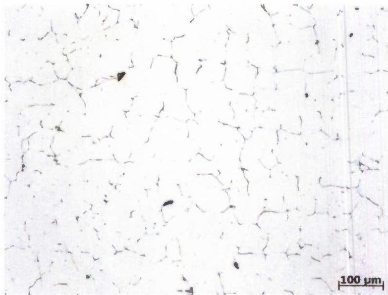
Figure 9 Micrograph of the 304 sample with a NiAl addition.
