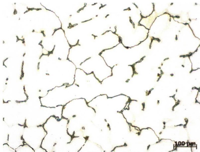
Figure 12 Micrograph of the HK sample with MgO powder addition.
