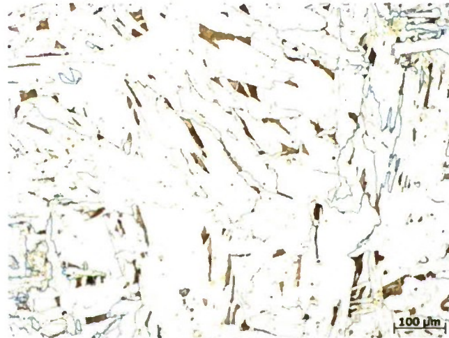
Figure 20 Micrograph of 1010 with no addition.
