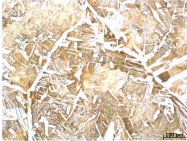
Figure 35 1030 steel with \text{La}_2\text{O}_3 addition.
