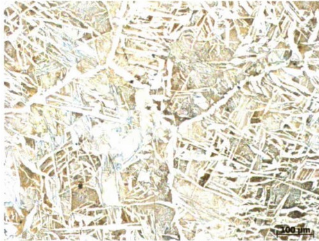
Figure 32 1030 steel with AlN addition.
