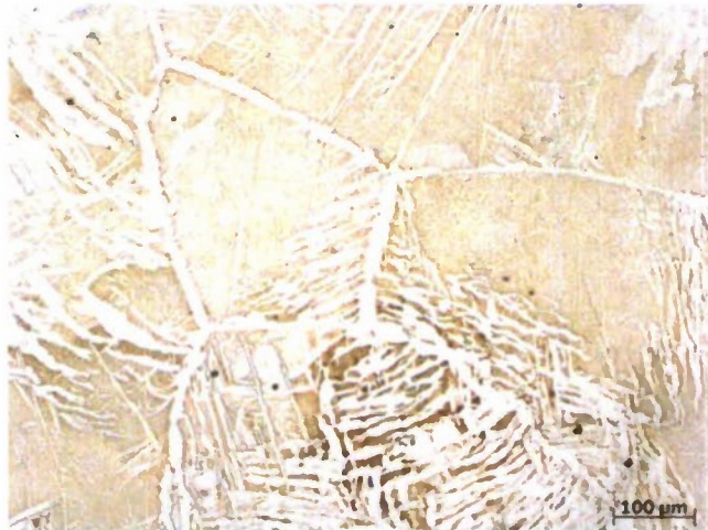
Figure 36 1030 steel with MgO powder addition.
