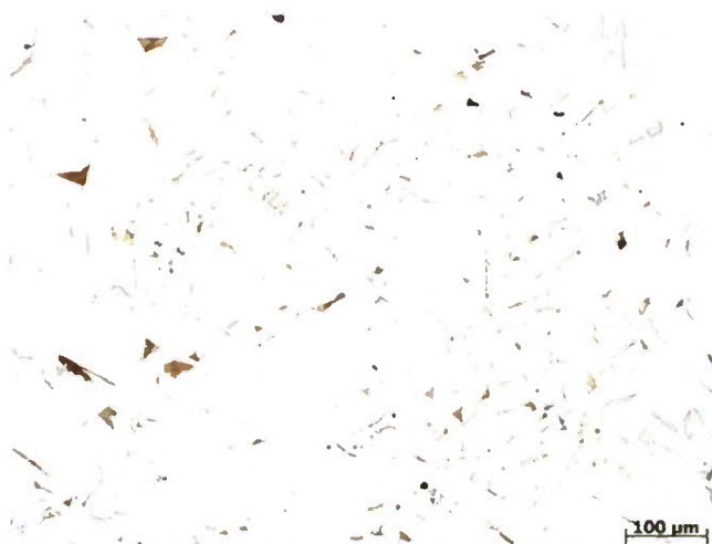
Figure 25 Micrograph of 1010 steel with TiN added.
