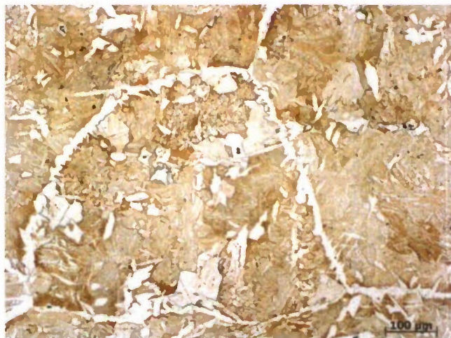
Figure 31 1030 steel with no addition.
