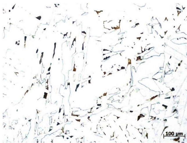
Figure 26 1010 steel with TiO 2 powder addition.
