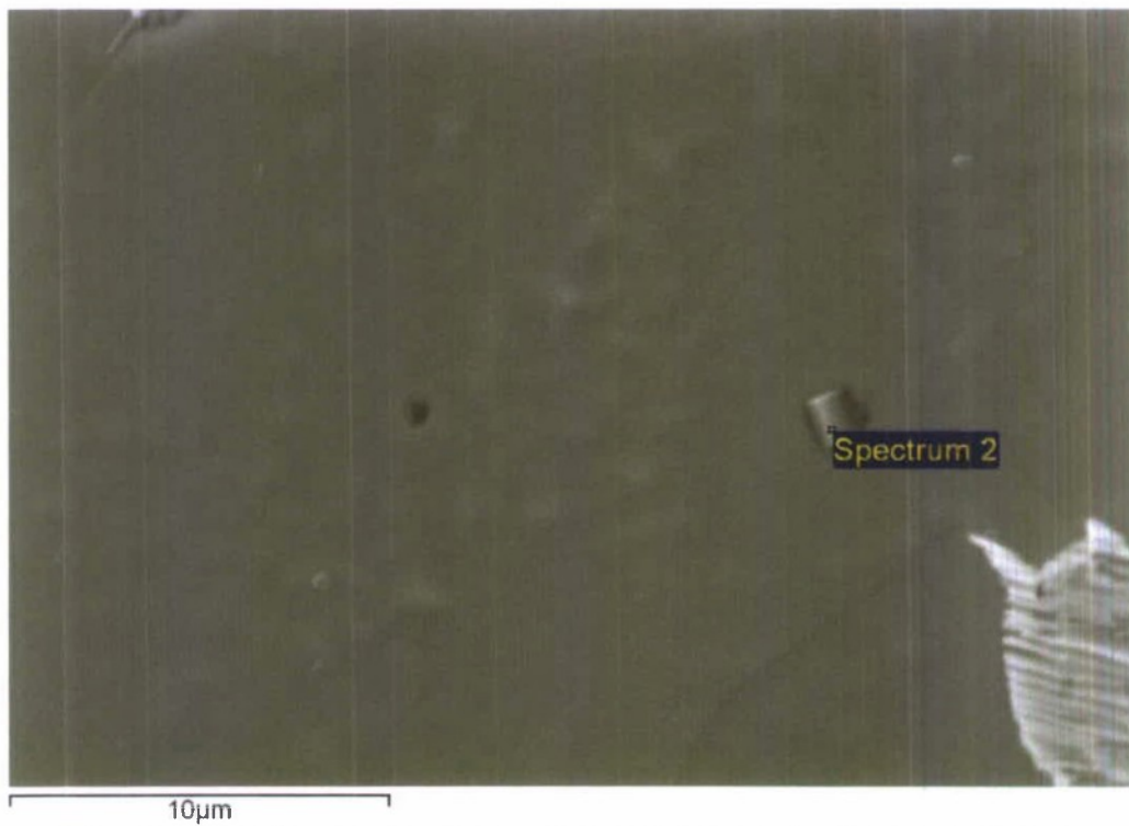
Figure 9 Particle near the center of a prior austenite dendrite in Sample 2.
