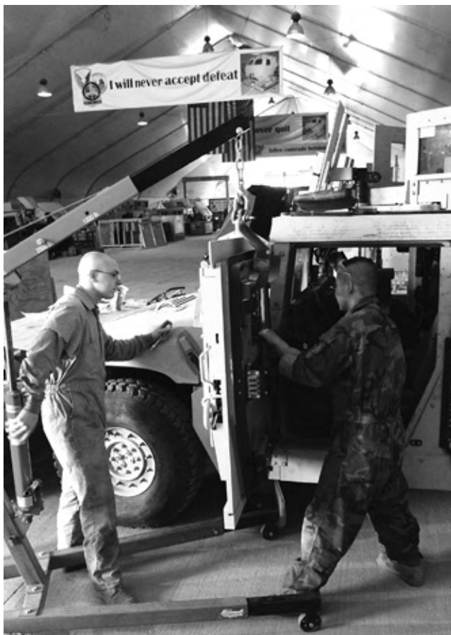
PFC Joshua Bullard and SGT Kang Hoon Lee, mechanics for the 122d Aviation Support Battalion, 82d Combat Aviation Brigade, use a hoist to install an up-armored door on a HMMWV, 25 May 2007, at Bagram Airfield, Afghanistan.
