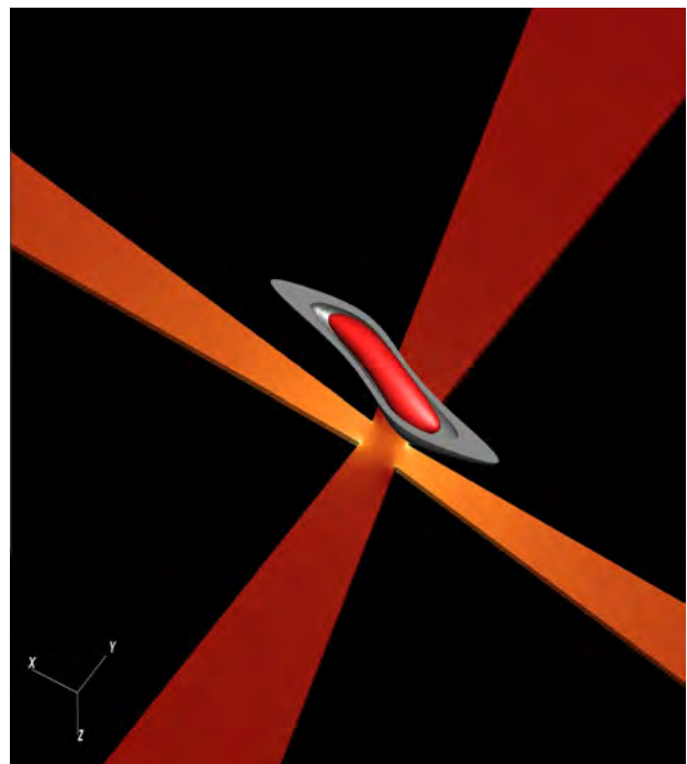
Figure 3: Peapod (1 hard shell in red, 2 more in gray, cut). This view provides insight into where the trap is and how the field changes around it.
