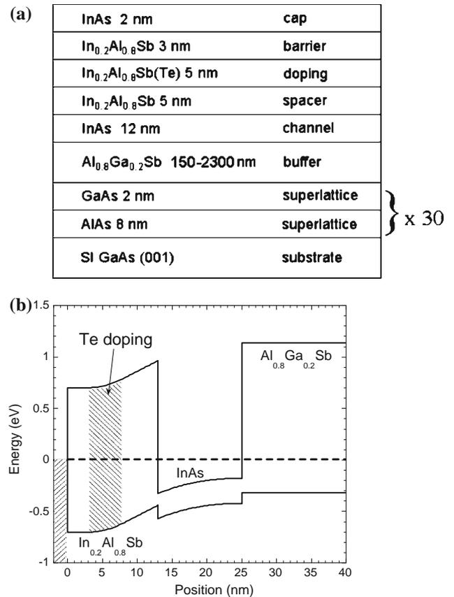
Fig. 1. Cross-section (a) and calculated band structure (b) of InAs quantum well heterostructures. The GaAs/AlAs superlattice is included for calibration.
