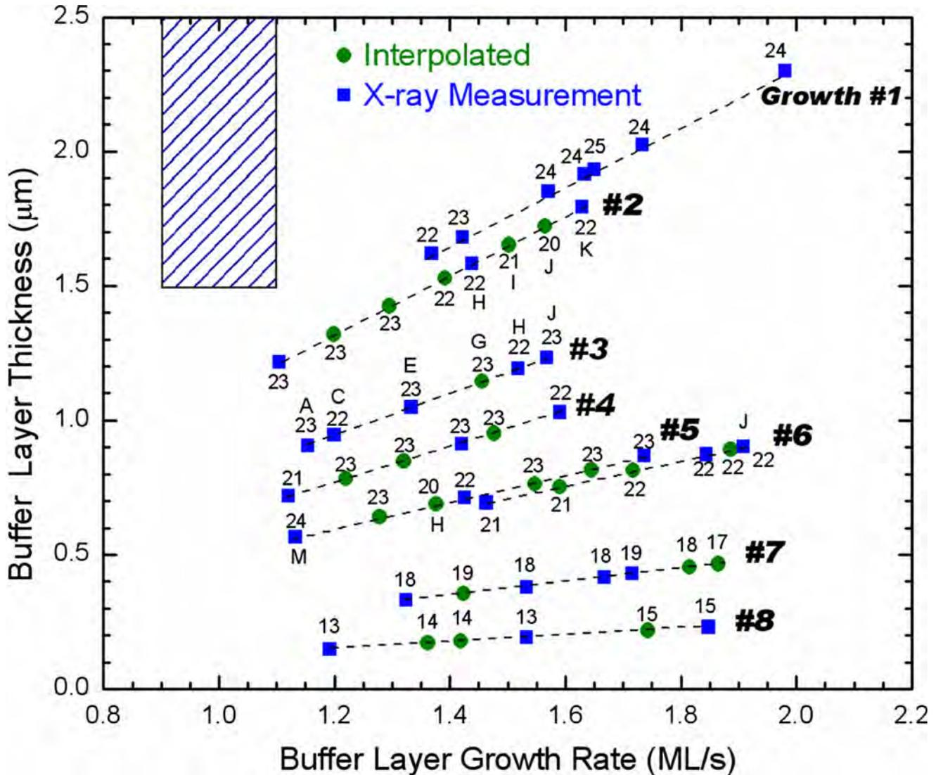
Fig. 5. AlGaSb buffer thickness versus growth rate; the *number* next to each data point is the room-temperature electron mobility ( $\times 10^3 \text{ cm}^2/\text{V s}$ ). Sheet carrier densities ranged from  $0.7 \times 10^{12}/\text{cm}^2$  to  $1.2 \times 10^{12}/\text{cm}^2$ . Samples discussed in the text are identified by *letter*. The *shaded region* represents the parameters used in most previous work.
