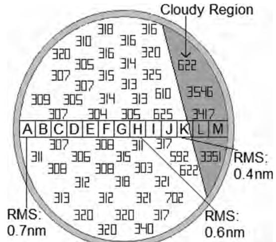
Fig. 2. Resistivity map of growth 3 in units of  $\Omega/\square$ . Thirteen  $5 \text{ mm} \times 5 \text{ mm}$  squares were cleaved and are labeled as samples 3A–3M. The substrate was not rotated during growth of the buffer layers, resulting in an AlGaSb growth rate which increased from left to right. The shaded portion on the right side represents a cloudy region with insufficient Sb flux. Surface roughness measured by AFM is indicated for three samples.
