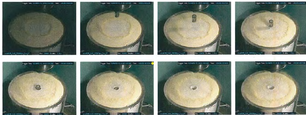
Fig.7 High-speed visualization of behavior of projectile during penetration. Frame rate; 20,000 fps, exposure time; 1 \mu s, impact velocity; 495 m/s, container; C.
