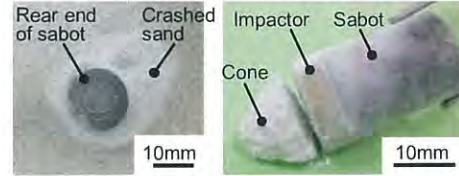
(a) Circumferential (b) Massive (ahead of projectile) Fig.12 Distribution of crashed sand.
