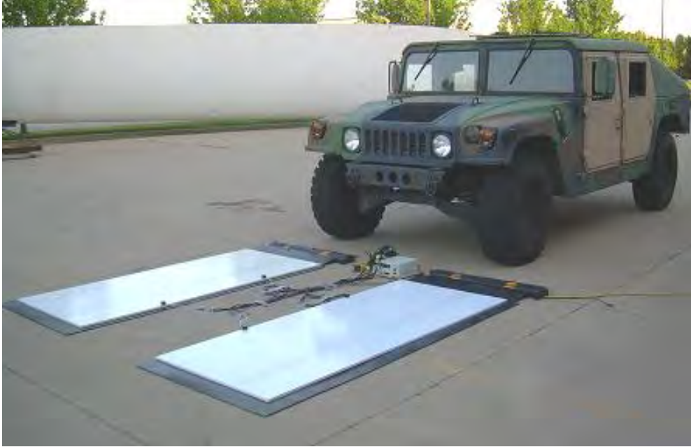
Figure 3. Photograph of extended diagnostic speed bump measurement configuration with rubberized cleat, measurement plates, sensors, and data acquisition system.
