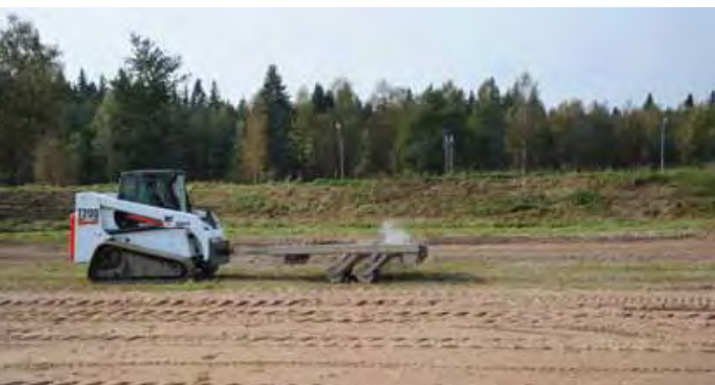
Image 8. SCAMP Roller with a Bobcat T-200 prime mover.
