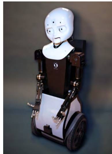
Fig 1. Octavia is an MDS robot with a 4-element microphone array mounted on the body, cameras in the eyes, and an SR3000 in the forehead.
