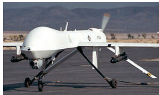
FIGURE 8: Rotax 914, a four-cylinder, four-stroke, 101-horsepower engine, the same engine type commonly used on snowmobiles, rotates the Predator's two-blade, variable-pitch pusher propeller [30–32].
