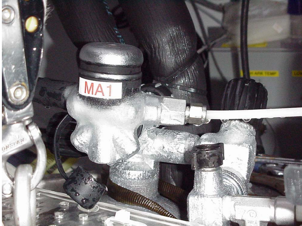
Figure 11. Typical First-Stage Icing (Mares Abyss attached to tank Manifold shown with intermediate pressure sensor adaptor and hose attached for testing)
