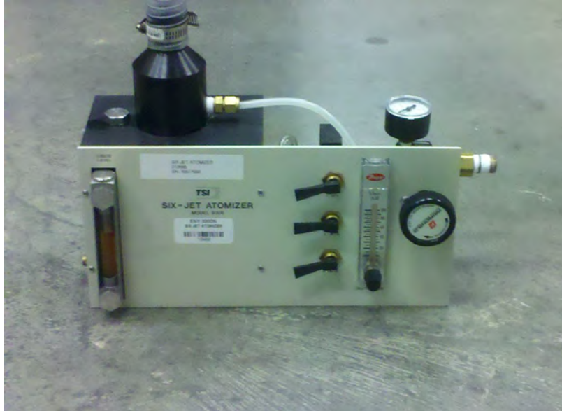
Figure 3.9: TSI Model 9306 Six Jet Atomizer
