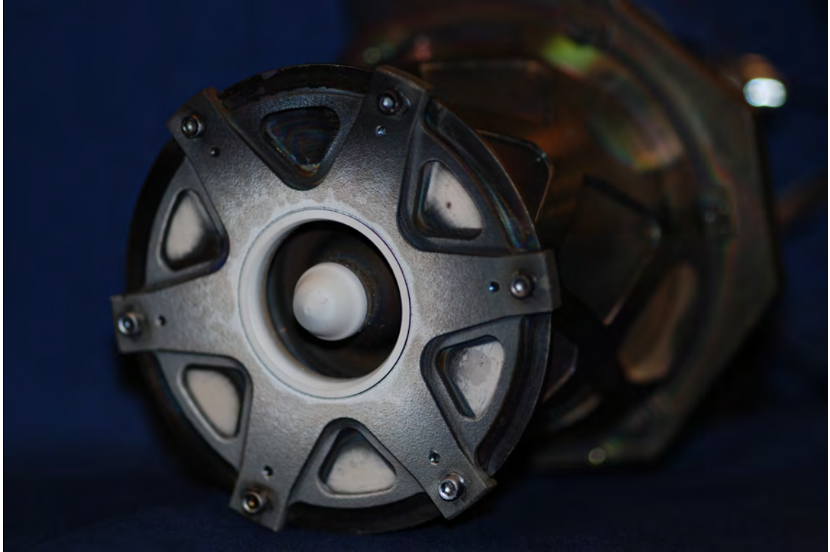
Figure 3.2: Photo of the BHT-200 Hall thruster.
