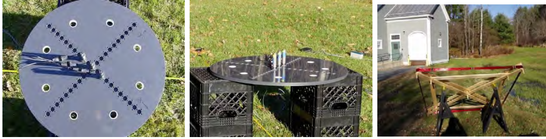
Figure 47. Receiver test fixture. Three vector magnetometers measure the center difference gradient values along two orthogonal axes (LEFT, CENTER). The receiver array is placed at various offsets from the transmitter to obtain localization estimates (RIGHT).
