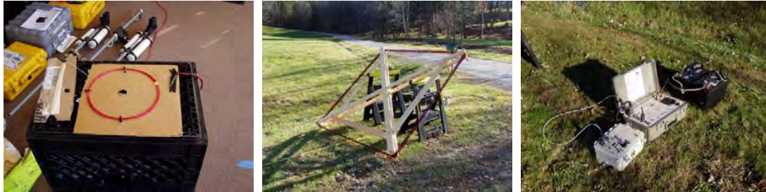
Figure 43. Dipole transmitters. Small moment transmitter (LEFT) for indoor testing; large moment transmitter (CENTER) for outdoor testing; Zonge International, Inc. ZT-30 transmitter source and XMT-32 transmitter controller (RIGHT).
