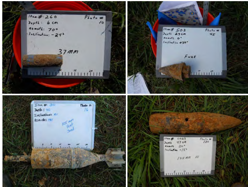
(b) Camp Butner. Clockwise from top left: 37 mm projectile, M48 fuze, 105 mm high explosive (HE) projectile, 105 mm high explosive anti-tank (HEAT) projectile.
